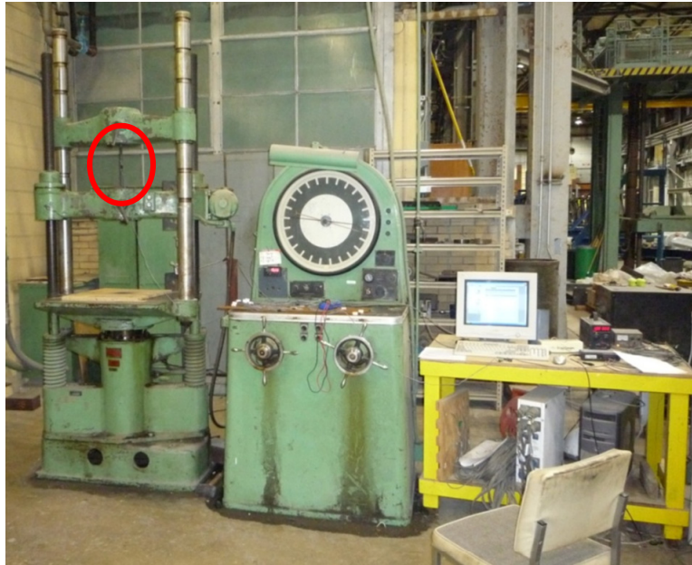
Figure 3.11 Reinforcing-bar tension testing in 60-kip test machine
