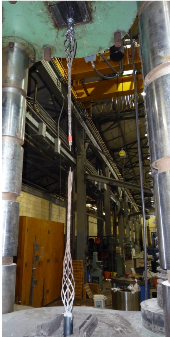
Figure 3.17 Typical strand failure mode
