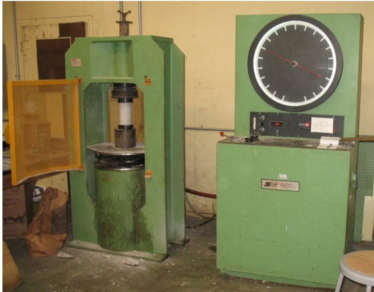
Figure 3.6 Cylinder compressive-strength testing
