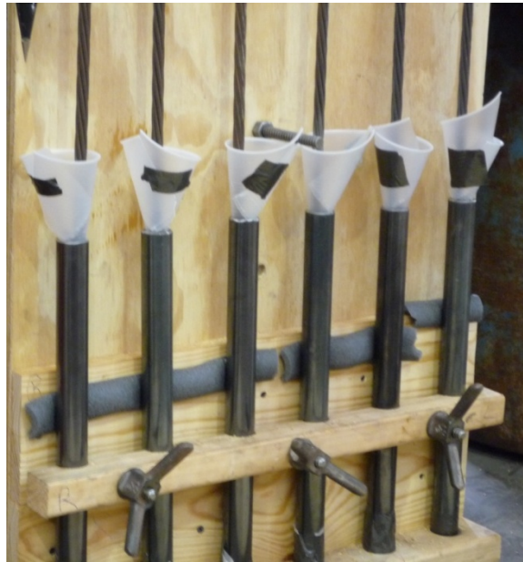
Figure 3.16 Strands epoxied into black pipe for tensile-strength testing
