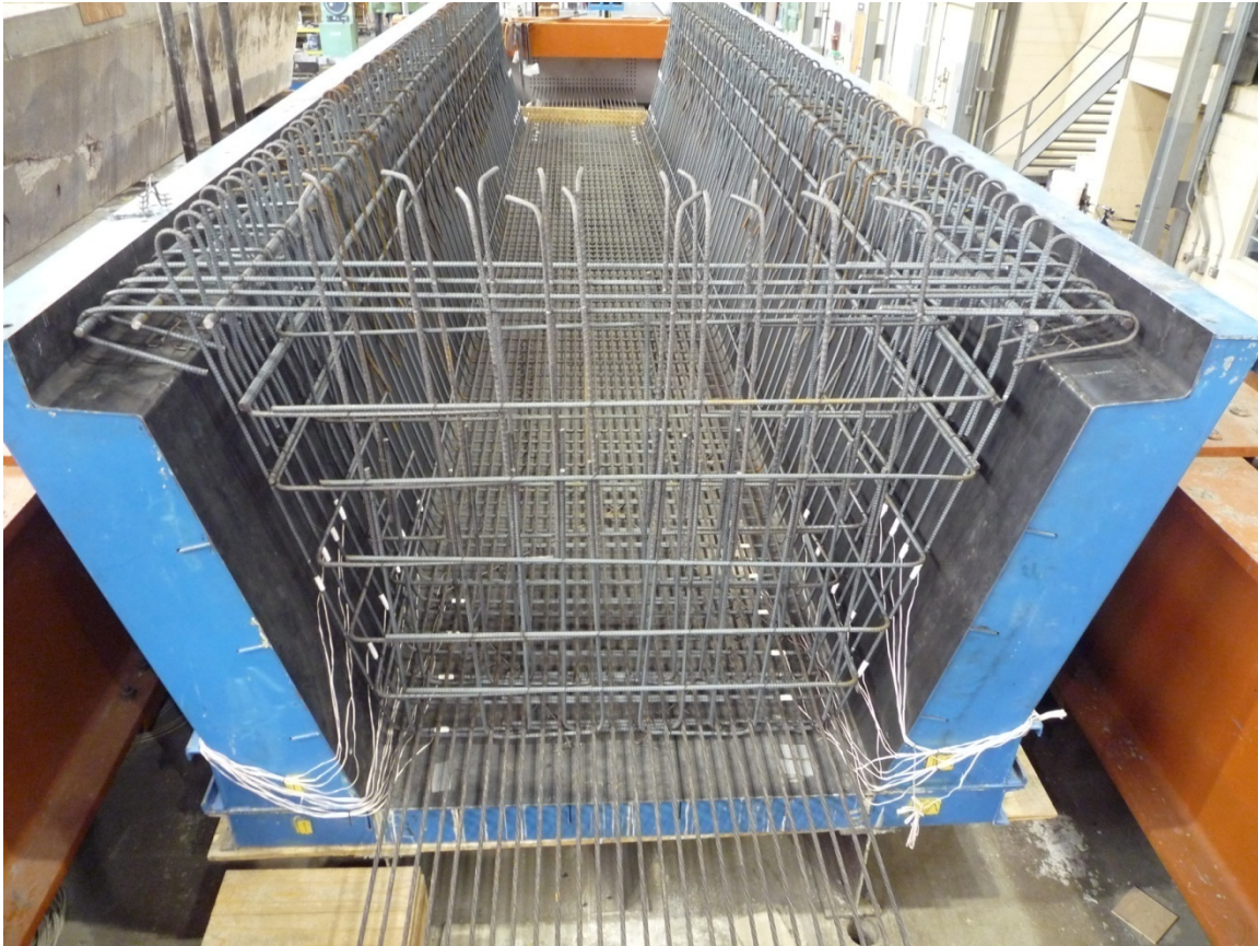
Figure 3.41 Strands installed, tensioned to nominal stress for instrumentation
