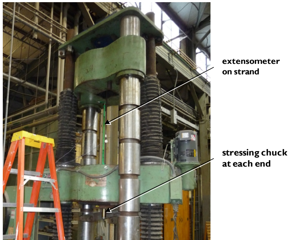
Figure 3.18 Setup used for Beam 2 elastic-modulus testing for strand
