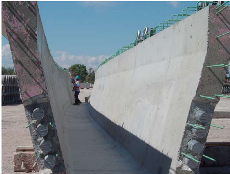
Figure 2.55 Curved pretensioned/post-tensioned Colorado U-girder (Endicott, 2005)
