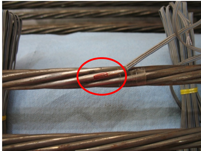
Figure 3.14 Typical strain-gage installation along pitched wire within strand (O'Callaghan, 2007)
