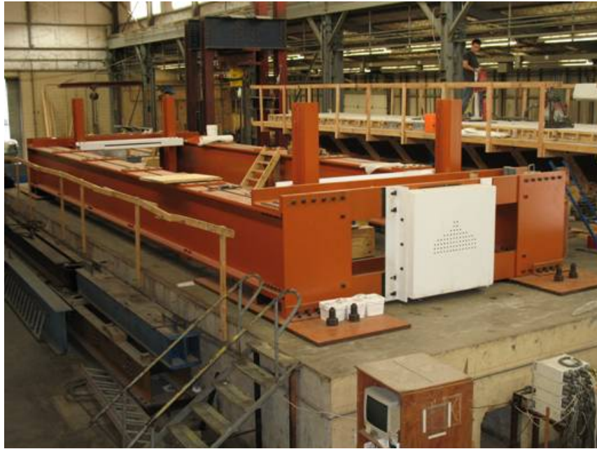
Figure 3.36 FSEL pretensioning bed (O'Callaghan, 2007)
