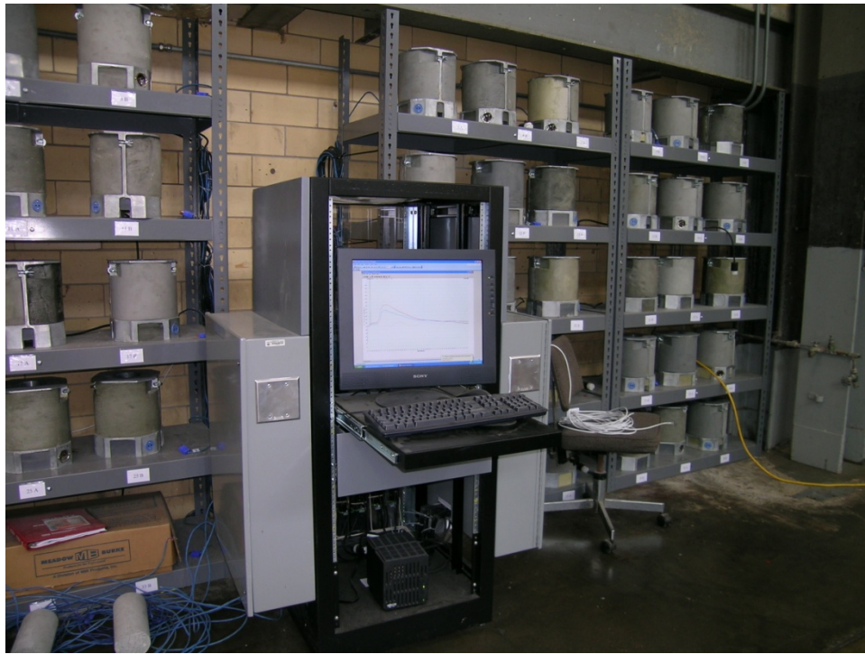
Figure 3.9 Sure Cure temperature-match-curing system (Tuchsherer, 2007)
